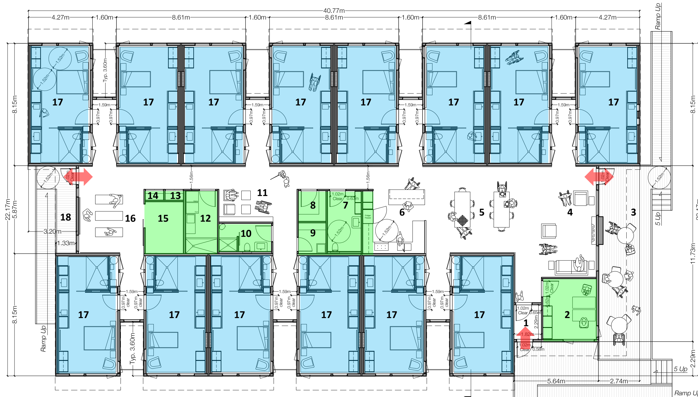
concept diagram of modular living units facing common vaulted space with central service areas and views to external courtyards
